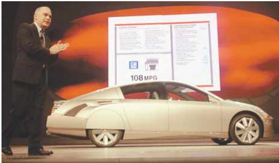
◆ FIGURE 18.7 ◆ The Precept, General Motors' New Diesel–Electric Hybrid, Gets 108 Miles to the Gallon
